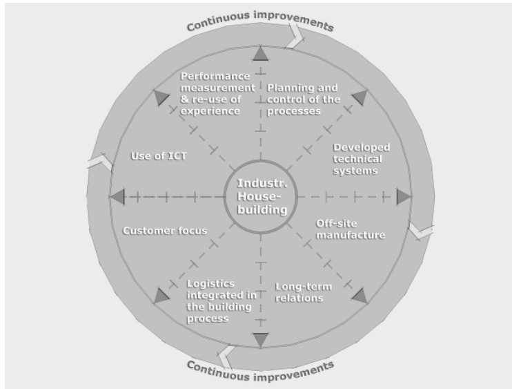
Figure 7.2 The Industrialised House-building Process Model, in which the areas can be developed to different levels.
