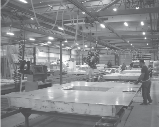
Figure 5.23 Production of a wall element at Finndomo's factory.
